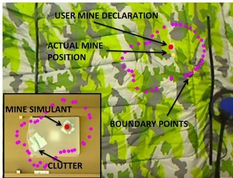
Figure 1: PETALS user interface (larger picture). Lower left hand corner shows underlying configuration of the detection task.
