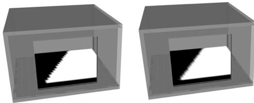
Figure 7 Shadow map before anti-aliasing (left) and after PCF (right).
